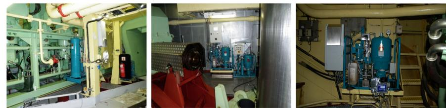
**Project background.** The project is based on a multi-sensor platform installed and running onboard three service vessels named "Achiever", "Assister" and "Attender". Each of these service vessels have oil filters and on-line multi-sensor platforms installed on expensive and critical oil lubricated systems such as azimuth thrusters, stern thrusters and cranes. The installations have been running since 2011 on Attender,
