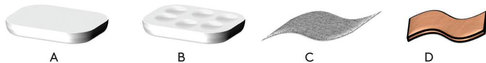
Figure 1. A simplified reconstruction of the main steps of the evolution of the supporting element: A. metal plate; B. metal plates with holes; C. metal-mesh; D. felt fabric, to be stiffened.
